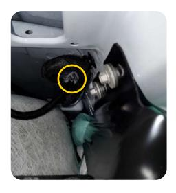
**STEP 2:**Unplug the OEM Cargo Lamp connectors and install the CL-FTC harness between the two
