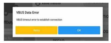
Note: The app will automatically disconnect from the device after attempting to connect for 1 minute and 30 seconds without receiving any data from the VBUS device.
