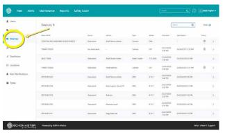
7. In the list of devices, find the device you just installed. Click the ">" symbol on the right side to open that device, and assign it to the vehicle you just added.
