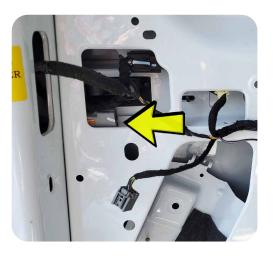
**STEP 2:** Install the P-BUA-TRANSIT CONNECT harness between the OEM connectors
