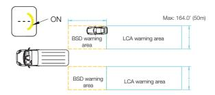
If a vehicle is in the LCA warning area and the overtaking time is less than 3.5 seconds, a first-level alarm will be issued (the color bar on the right side of the display will be ON)
