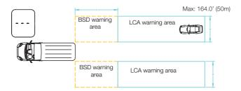
If a vehicle is in the BSD warning area, a first-level alarm will be issued (the color bar on the right side of the display will be ON)
