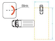
When an obstacle on the left side enters the warning area, the color bar on the left side of the display blinks and beeps twice.
