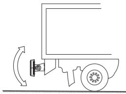
A. The sensor bracket is fixed on a horizontal plane and the vertical installation angle is adjusted through the installation bracket.
