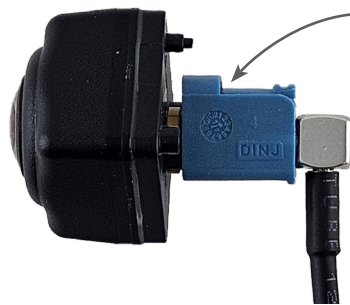
Fully Seated Connection
