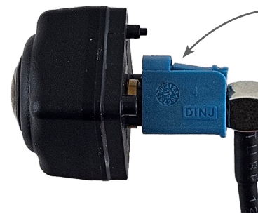
Not Fully Seated Connection
