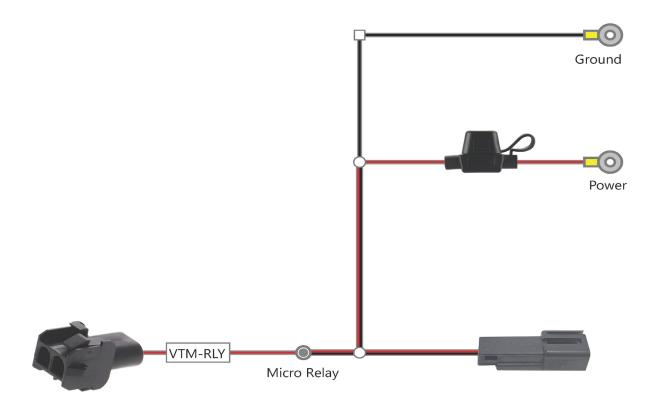
VTM-RLY Output connects to P-VTMxxx harness for vehicle lighting
