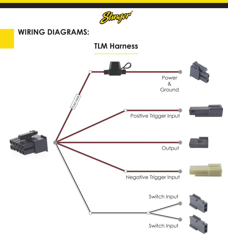
If necessary, connectors may be removed for hardwire applications.
